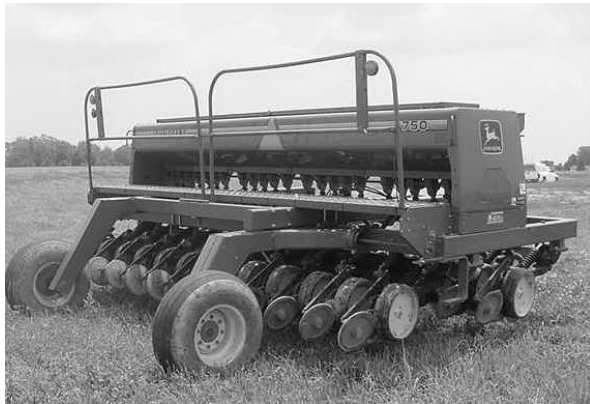
J.D. 750 Drill with grass seed attachment has 7 1/2" row spacing.
